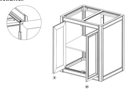
18.) Screw panel (F) into the end caps with the provided 4 x phillips head screws.
