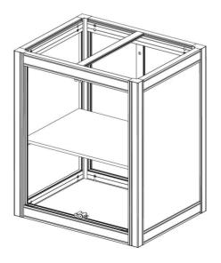
16.) Insert the door (M) into the white pivot brackets. Slide the door to the left and tighten top and bottom pivot brackets using a phillips head screwdriver.
