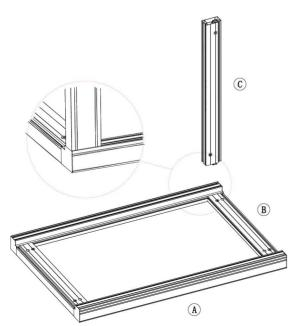
4.) Attach Horizontal Cross Profiles (2 x D) to (A & B) and lock into place.
