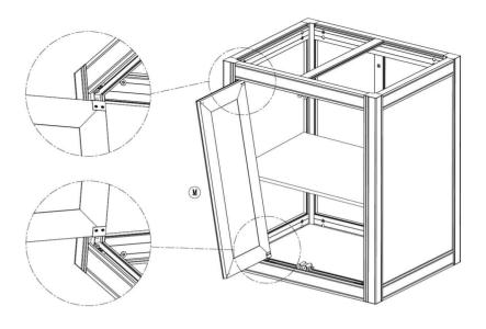
17.) Repeat step 16 with door (M1). Slide the door to the right and tighten top and bottom pivot brackets using a phillips head screwdriver.
