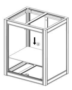
13.) Insert shelf locks (4 x N) into the smallest channel on the profile.  $\bigcirc$
