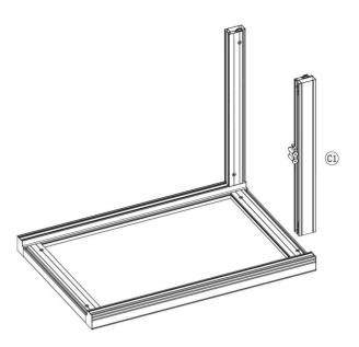
2.) Attach Top or Bottom Rear Profile (C) to (A & B) and lock into place. Make sure the profiles line up with the end caps.
