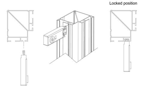
To securely lock each profile into position, insert the supplied hex torque wrench into the tension lock and turn clockwise.
