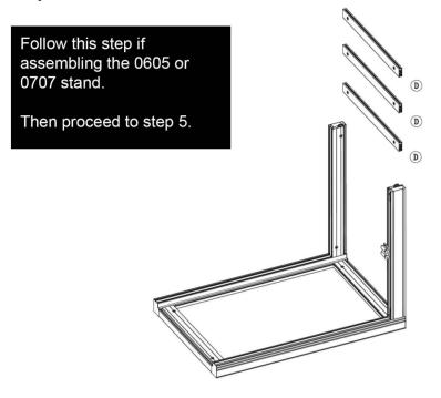
5.) Attach Top Profile (C) to the top of (A & B) and lock into place.
