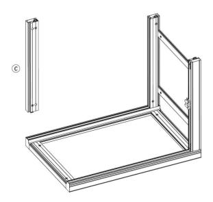
6.) Attach Top Front Profile (C2) to the top of (A & B) and lock into place.
