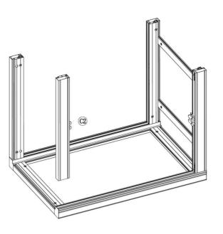
7.) Attach Horizontal Cross Profiles (D) between (C and C2) and lock into place.
