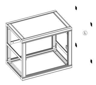
11.) Flip stand onto its base and make sure all profiles are locked and stand is level.
