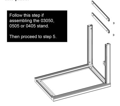
4.) Attach Horizontal Cross Profiles (3 x D) to (A & B) and lock into place.
