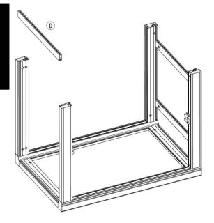
7.) Attach Horizontal Cross Profiles (2 x D) between (C and C2) and lock into place.
