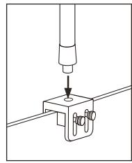
A4. Screw gooseneck into the gooseneck base
