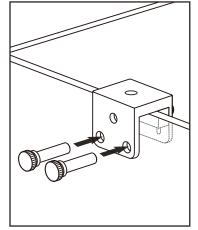
A3. Screw thumb screw onto gooseneck base to secure base to aquarium
