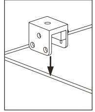
Insert plastic stepper into gooseneck base and secure A2. Place gooseneck base onto aquarium.
